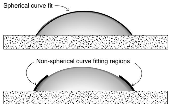
Figure 6. Spherical and non-spherical fitting regions.
