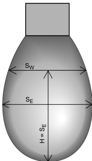
Surface tension is derived from drop shape. Given fluid density, the value of  $S_W / S_E$  is an entry into a lookup table which yields surface tension.
