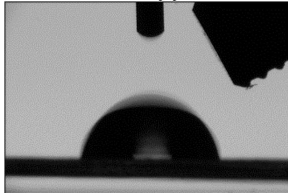
Figure 1. Initial contact of droplet on paper.
