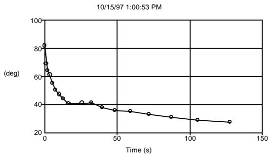
Figure 3. Contact Angle of Water on Paper.
