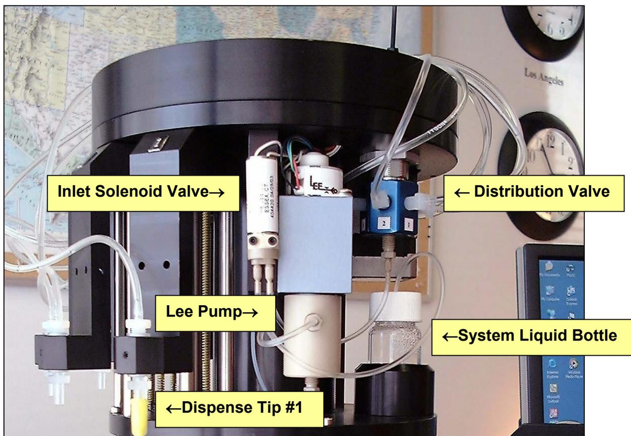
Liquid system. The Outlet Solenoid Valve is not visible; it is hidden on the far side of the block behind the Inlet Solenoid Valve.
