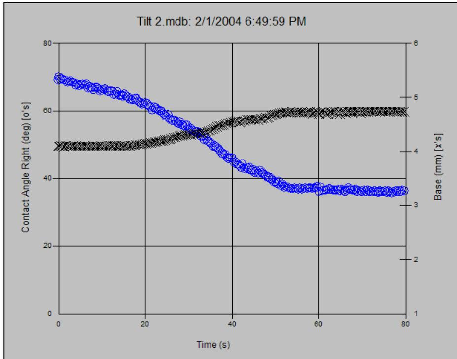
The base width curve is the same as in the previous graph. The uphill receding angle starts high and then decreases until it reaches a plateau around 53s.
