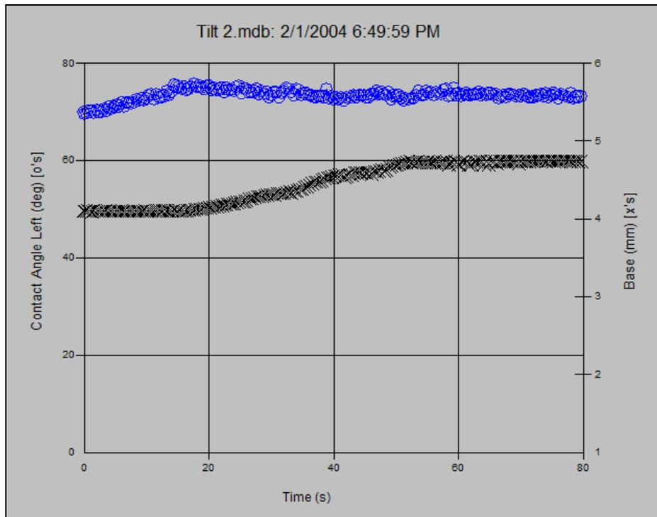
Upper curve is the downhill advancing angle. It reaches a more or less stable plateau as the lower base width starts to expand at 17s. This expansion is the motion of the wetting three phase line.
