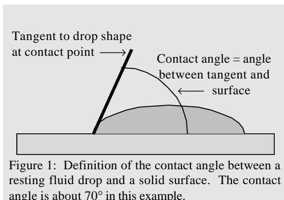
Figure 1: Definition of the contact angle between a resting fluid drop and a solid surface. The contact angle is about 70° in this example.
