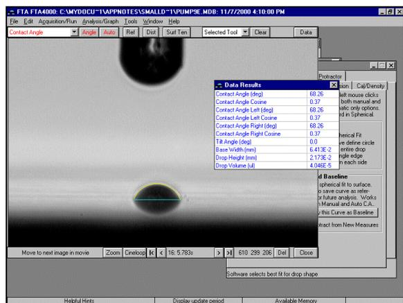
Five drops were placed on the anodized aluminum sample. The table lists the sessile drop volume and the initial contact angle. These drops are so small they evaporate in less than 1 second. The contact angles are consistent with microliter sized drop angles placed on the same sample.
