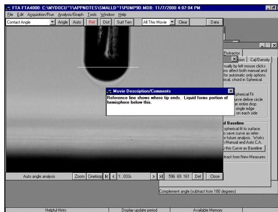
It is touched off in the following images. When the liquid touches the surface, it forms a complex capillary between the surface and the tip, with a small radius of curvature so no great pressure drop occurs and no flow results. The period the tip is low is 0.167s, from the first to the second image. The capillary remains essentially constant.
