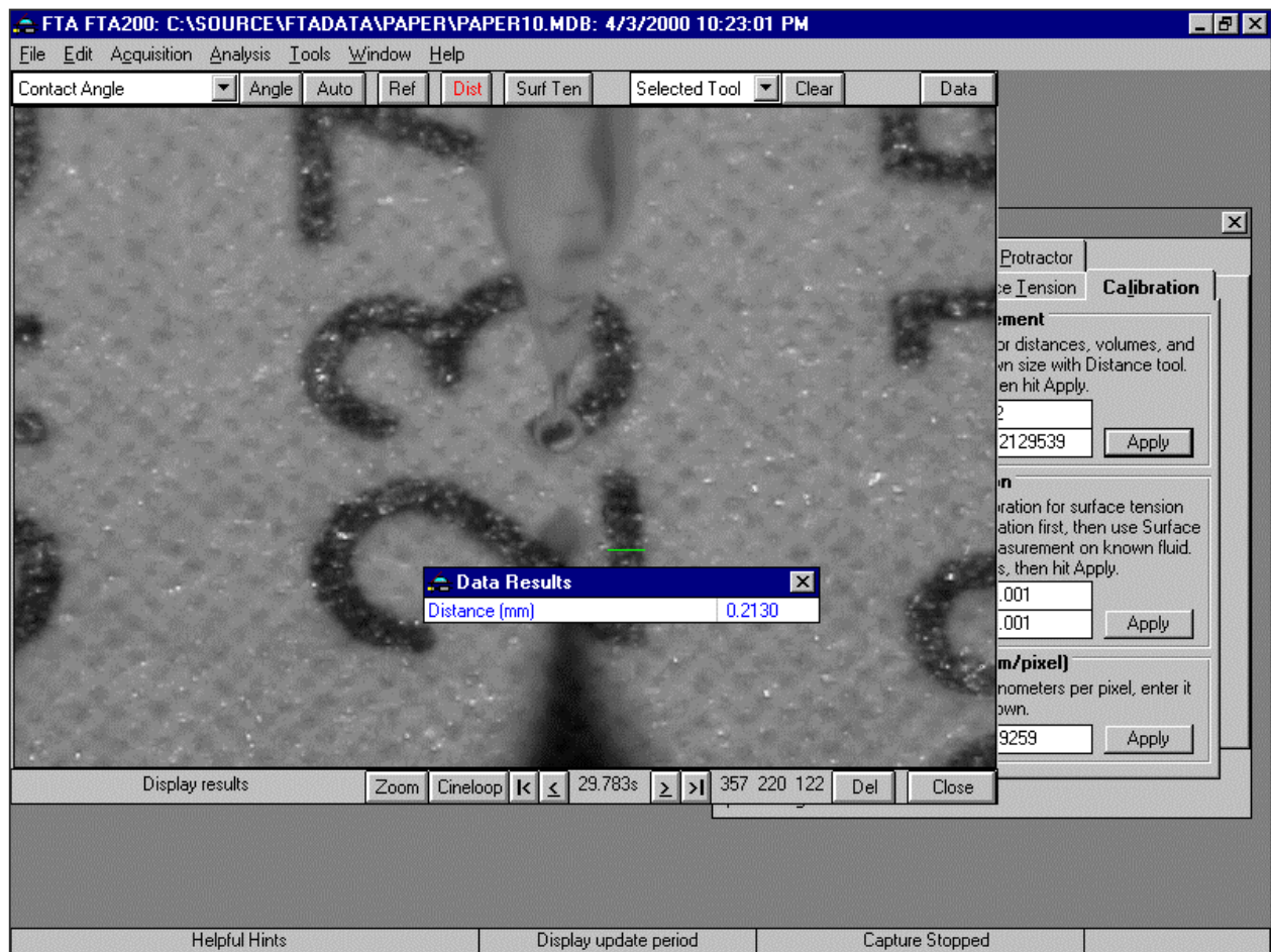
Figure 1. Drop on end of glass needle, ready for deposition.
