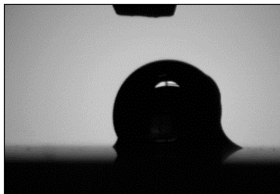
Figure 6. PtAg film with solder ball and flux.
